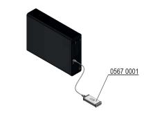
Connect using the connection cable, the humidity/temperature measurement system to your PC.
