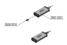
Connect the digital humidity/temperature probe HYT 131 (Item No.: 0636 0016) with one of the existing RJ12 sockets of humidity/temperature measuring system (Item No.: 0567 0001).
