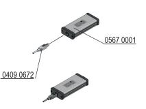
• Connect the humidity / temperature measurement system (Item No.: 0567 0001-10) with the connection cable (Item No.: 0409 0672).
